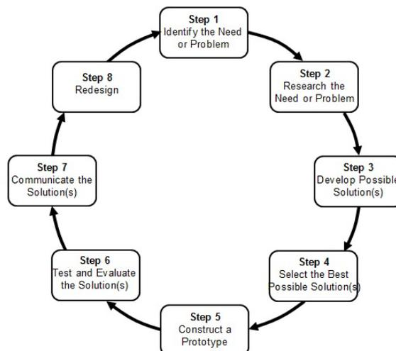
Figure 2. The Engineering Design Process
